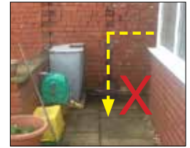
Check that the hot tub can clear a 90° turn
