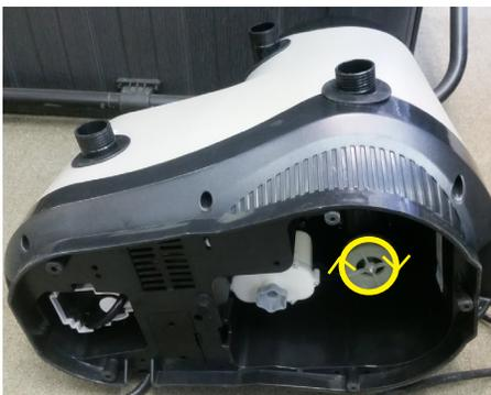
• Also, ensure that the Blower Check Valve, located under the Control Pack, is tightly secured. These can sometimes become dislodged during shipping, and cause tub malfunctions.
