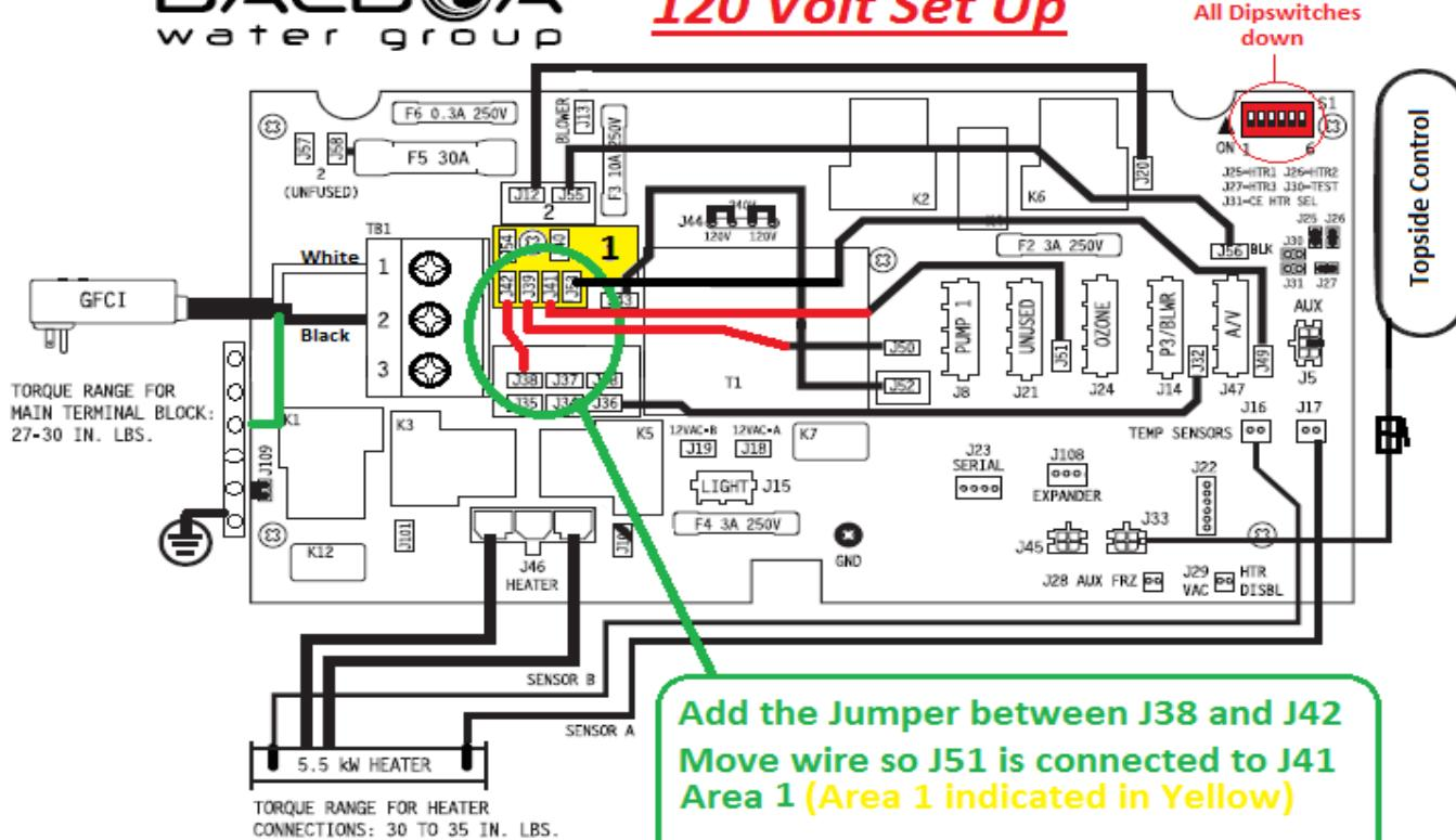
\*\*PUMP 1 AND OZONE MUST BE WIRED TO 120VAC WHEN SYSTEM IS
